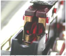
figure 2: Correct position of the contact sheets
