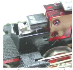
figure 4: The component in its correct position after being pushed in completely
