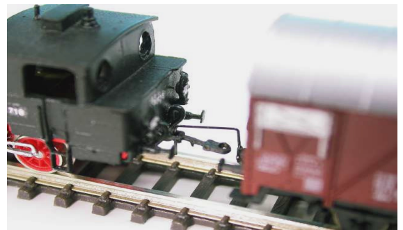
figure 3: Coupling with a newer coupler hook
