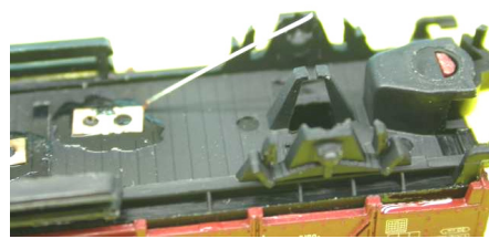
figure 8: The correct position of the current collector without the axle
