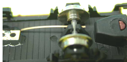
figure 7: The uninsulated side – always on the side where the current collector is located. Very important!
