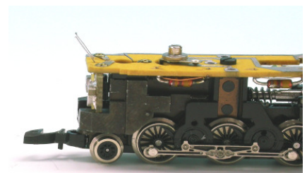
figure 6: Use your fingers to push the component towards the back.
